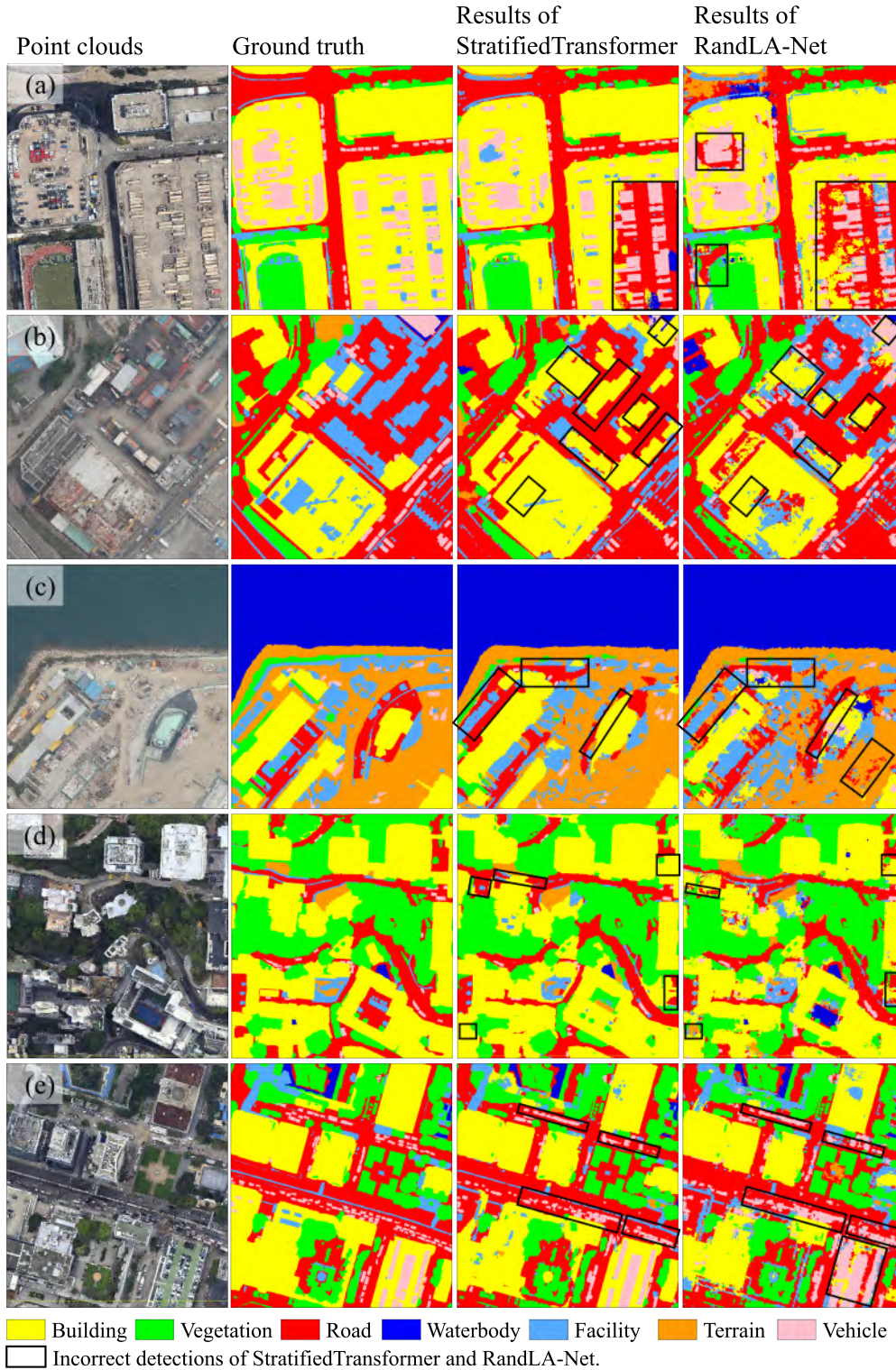
Figure 5: Typical errors of StratifiedTransformer and RandLA-Net on HRHD-HK. (a) Confusion between large-size building roofs and roads; (b)-(d) confusions between facility and building, roads and terrain, and roads and building podiums; (e) poor detection of vehicles.
